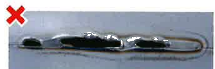
Burn-through caused by excessive heat input
