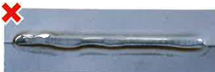
Meandered weld bead due to heat input shortage.
