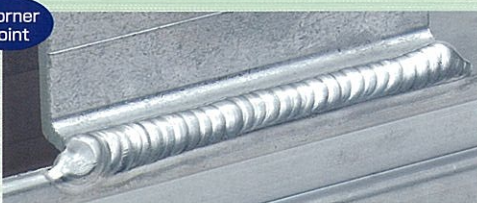
Welding current: 130A, AC frequency: 150Hz Welding speed: 25cm/minute, Plate thickness: 3mm (A6063 + Casting)
