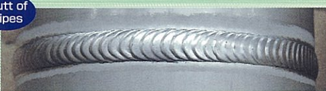
Pulsed current 200A, Base current 20A, Pulse frequency 2Hz AC frequency: 150Hz, Welding speed: 20cm/minute, Plate thickness: 4mm (A6062)
